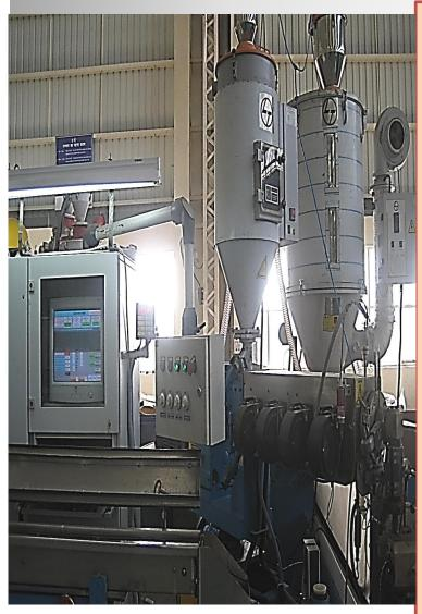
Insulation process is being carried out in very sophisticated world class extruders and dust free environment.
