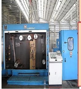
In line annealing/softening is being processed by controlled Induction heating thus high level of % annealing is being achieved which ensures approx 2% extra retaining of conductivity.
