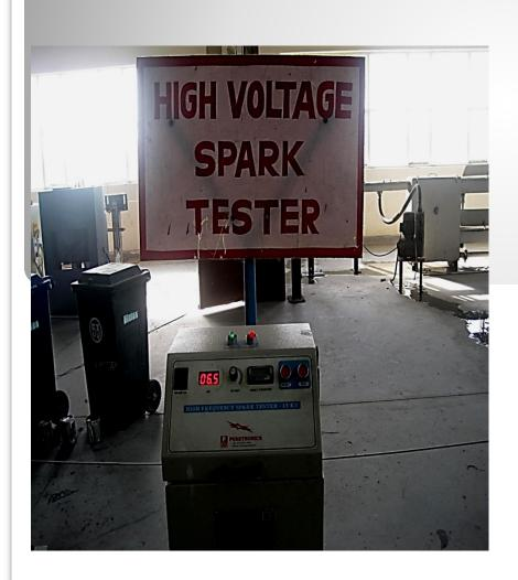
Insulated wire passes through on line High voltage test at 6000 Volts,
